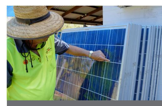
Inspecting cheap panels, that failed after 3 years and were pulled off the roof. The consumer was unable to claim against the manufacturer who had left Australia.
